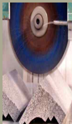
Diamond Saw Cutting
