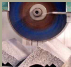
Diamond Saw Cutting
